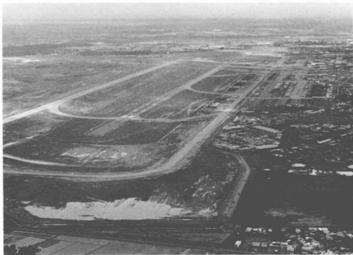
11. Tan Son Nhut Airfield. Located at the northern edge of Saigon. This 3,500-acre base was originally built by the French Army. A 10,000' concrete runway with connecting taxiway and warm-up apron were added. Tan Son Nhut was jointly used by commercial airlines and military aircraft of South Vietnam and the United States. At its peak, Tan Son Nhut had more daily takeoffs and landings than any other airfield in the world.
